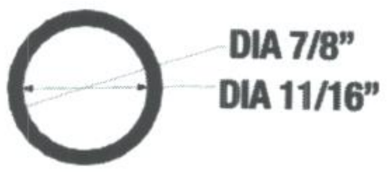
7/8" OD 14GA STEEL TUBING (STANDARD STEEL FRAME)
